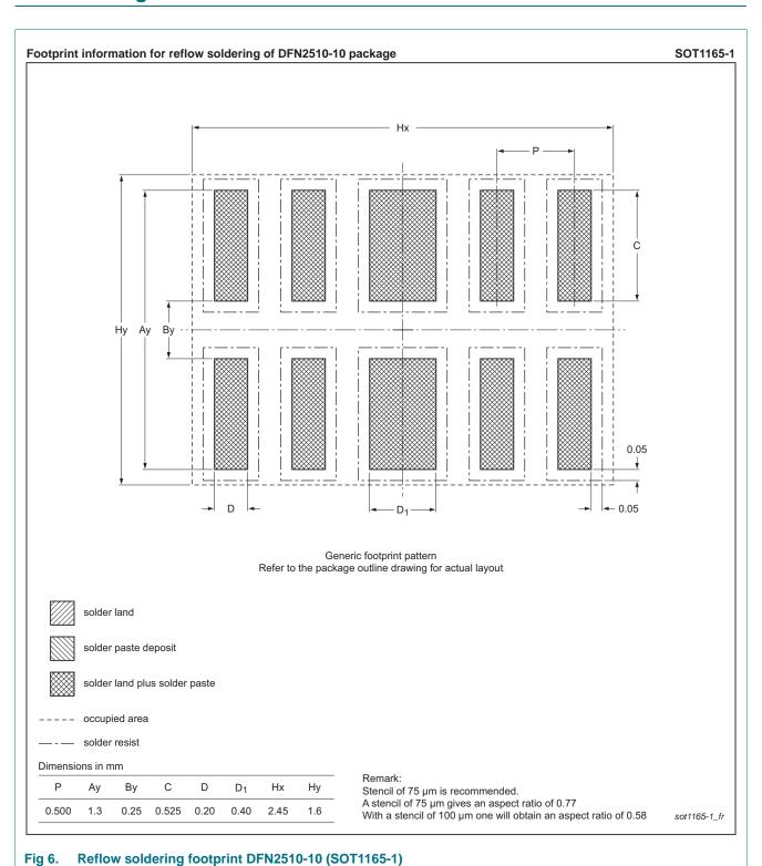
rig 6. Renow soldering rootprint of N2310-10 (3011103-1)
